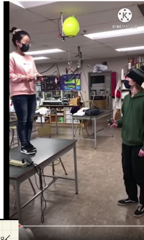
Acoustic stopwatch to measure free fall time
